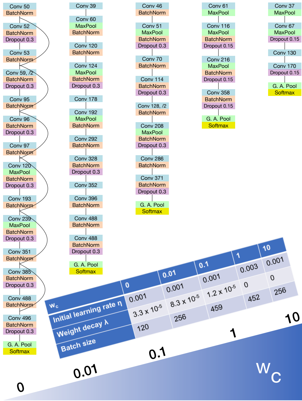
Figure 7.6: The best configurations found by DnC for CIFAR-10 augmented for w_c = [0, 0.01, 0.1, 1, 10] from left to right. Each configuration shows the architecture with input at top and output at bottom. Blue rectangles denote convolutional layers with their c value and stride shown as ‘/2’, orange BN, purple dropout with drop probability, green pooling, and finally yellow denotes the softmax classifier. The table at the bottom shows the best training hyperparameter values obtained.
